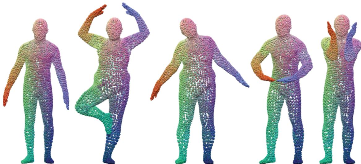
Colors transferred from reference to query shapes using correspondence learned with ACNN (similar colors encode corresponding points)
